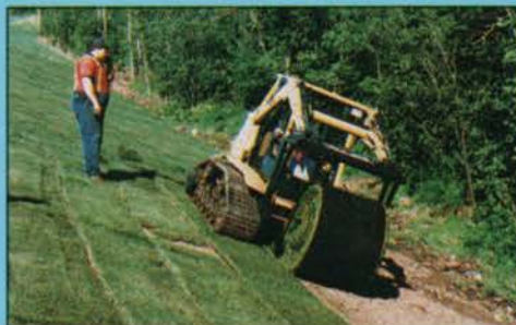
Low ground pressure allowed this Posi-Track to lay 115' sod rolls out in front, on a side hill.
