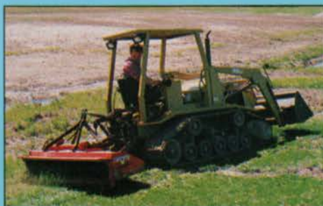
The loader attaches to either end, and the seat is reversible. The 3-point hitch makes good use of the standard PTO shaft.
