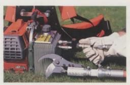
With the aid of a special adapter the 250PS can also be combined with shaft-mounted loppers.
