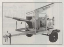
single-handle bar control for a 360-degree horizontal swing, 35-hp engine, vernier type throttle with weatherproof boot and twopiece load tray that extends for operator convenience.
