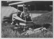
sides. Self-leveler automatically tilts to keep the operator's station level, as well as the engine for proper lubrication. Weight distribution remains constant over the drive wheels. Other features include dual hydrostatic drive, power-assist wheel lift for zero-turning radius and one-hand steering for total control of speed and turns without using foot pedals. **Circle 134 on reader service card**
