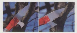
This pole saw with bark knife has a curved blade with a hook at the tip. The hook can be used to attach a line with which to apply greater pressure during cutting. The bark knife is used to cut the bark before you begin sawing, to prevent it flaking off when the branch falls. The blade is impulse hardened. The telescopic shaft can quickly be extended from 8 to 16 feet.
