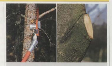
When cutting branches it is often necessary to make several cuts to prevent splitting. The cutting head of the 250PS and 235P is jointed so that you can easily adjust it to the desired angle. When you cut a branch close to the trunk it is important to leave the collar. This is a natural defense feature of the tree and helps the wound heal over.
