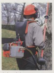
Lightweight harnesses are very easy to put on and spread the weight evenly over a large area. The broad hip belt carries most of the load and allows you to move your arms freely. Engines are well insulated and mounted on a generously padded, ventilated back support to eliminate irritating vibration.
