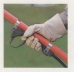
On both the 250PS and 235P the throttle control can be positioned anywhere along the shaft. This ensures a comfortable working position and saves you having to move your feet to reach different heights.
