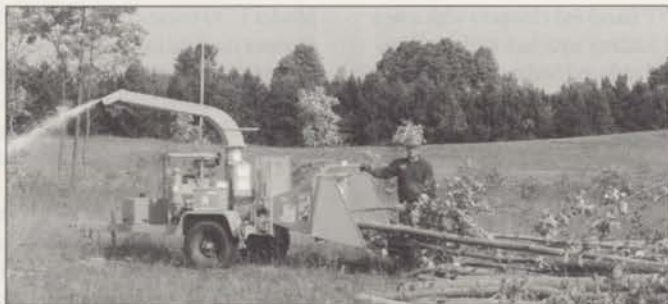
Wider feed openings accept large branches and save on labor. Photo credit: Bandit Industries
