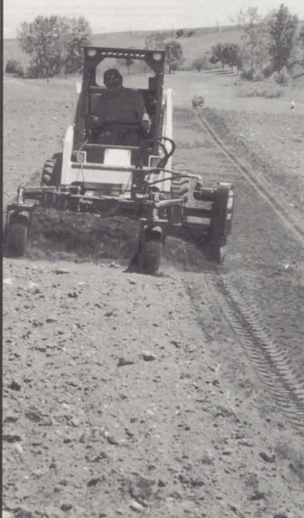
Harley Power Box Rake models are available for skid steer or tractor mount.
