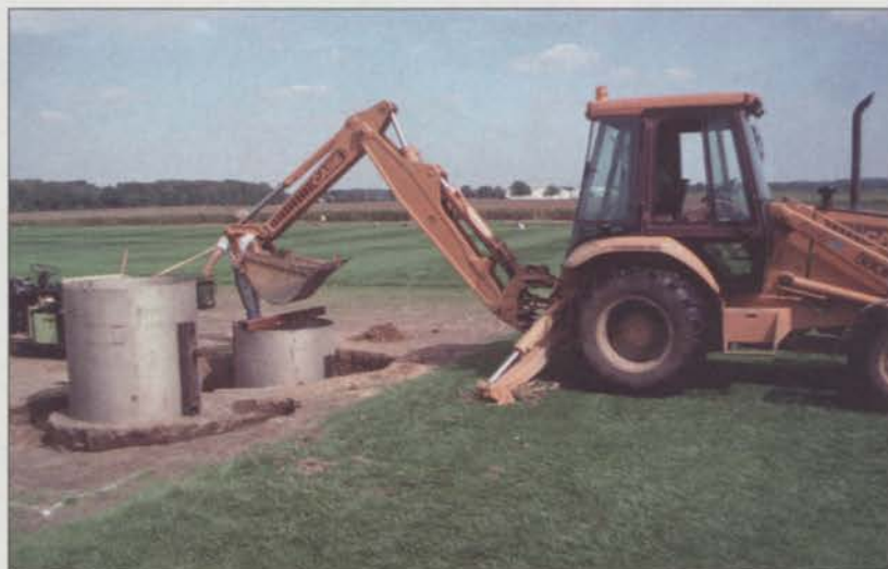
Before starting a series of fertilizer applications, Michigan State University researchers install lysimeters to monitor nitrate leaching over a three-year period. Photo: Branham
