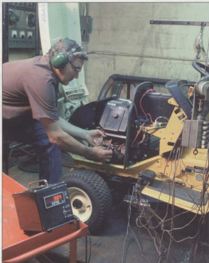
Kohler's application engineering laboratory includes the 'hot room,' where engines are tested at simulated high temperature conditions.
