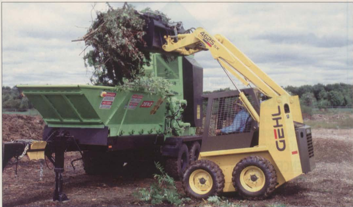
Hard-working skid steer loaders perform a wide variety of specialized landscaping tasks from grading to snow removal.
