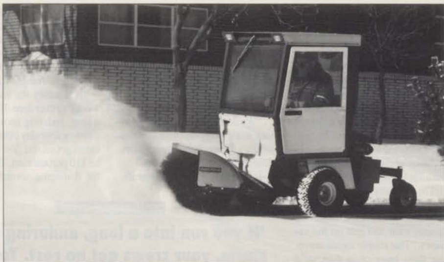
Grasshopper's 48-inch Sweepster rotary broom clears snow at a 30-degree right discharge.
