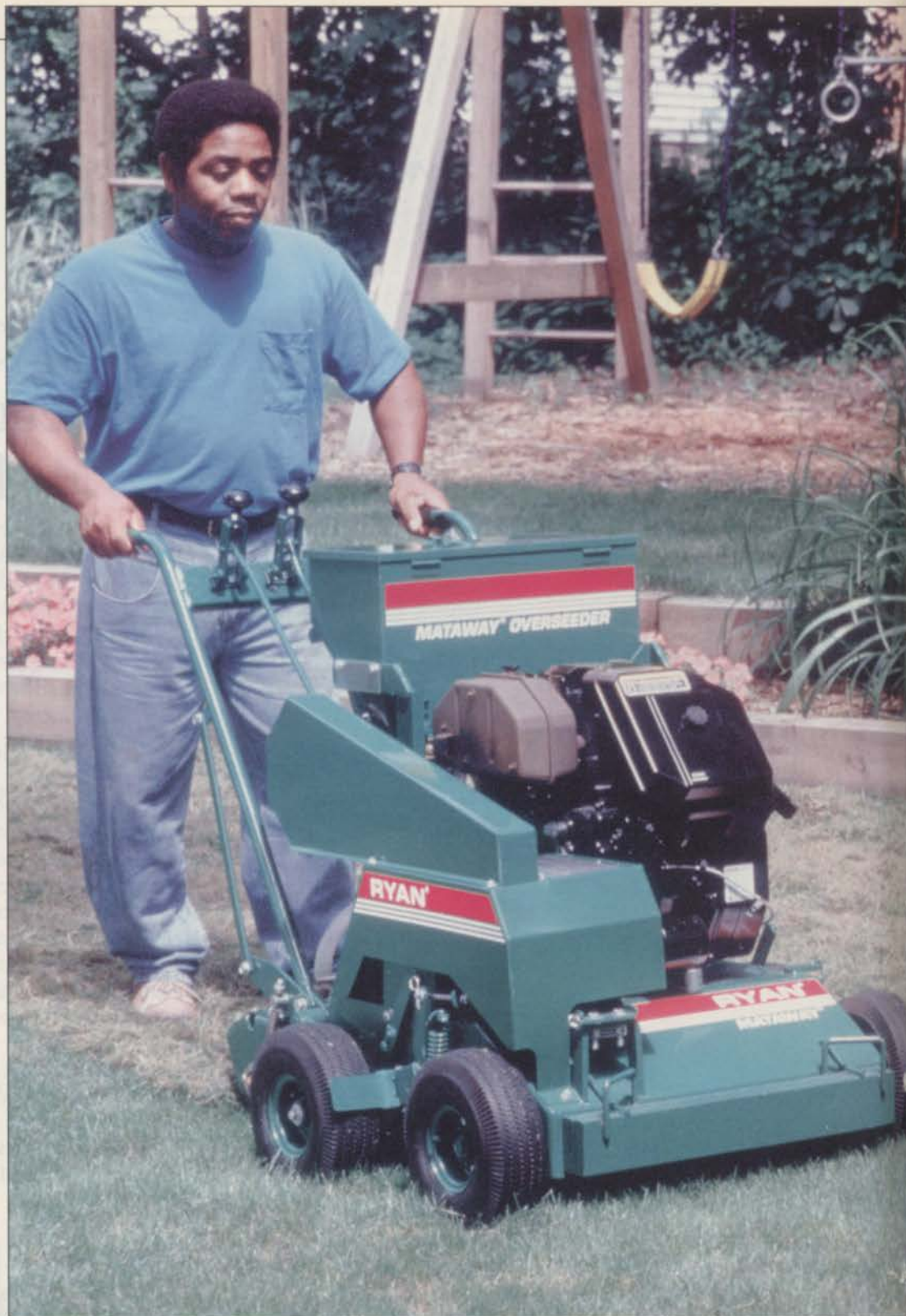
Large overseeders cut through thatch and apply seed within the open slit. Photo: Ransomes.
