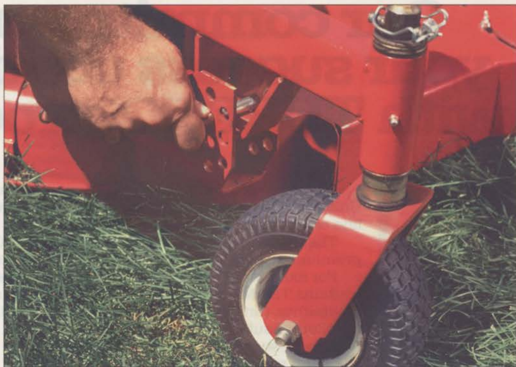
Mowers today are increasingly employing mowing height adjustment capabilities. Photo: The Toro Co.
