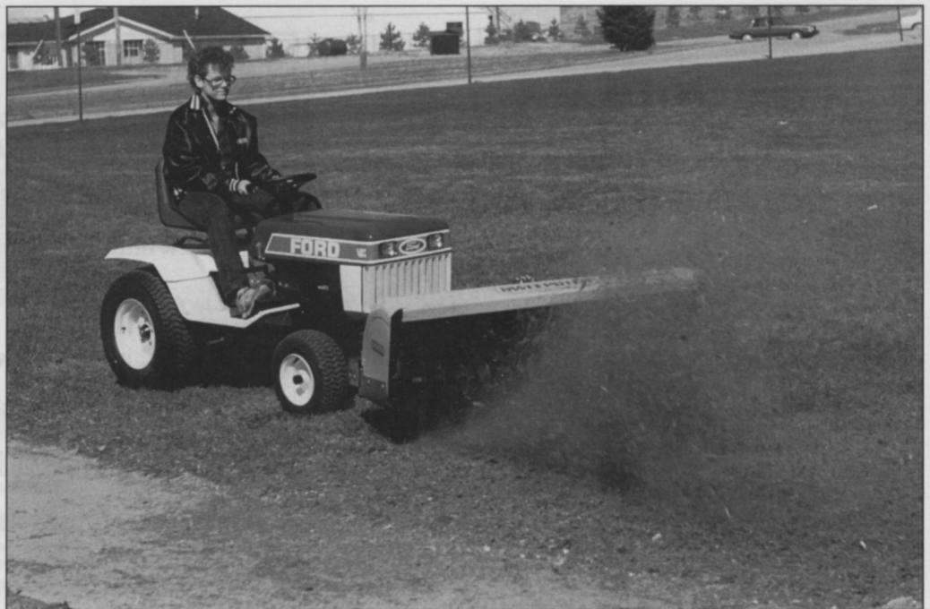
Sweepster's model CFM, mechanical-drive sweeper mounts to commercial riding mowers to clean away debris without damaging turf roots. The brush's angle changes 30 degrees left or right.
