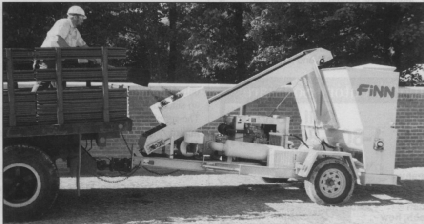
The flow rate with the Finn spreader is said to be 70 percent faster than if done by hand.
