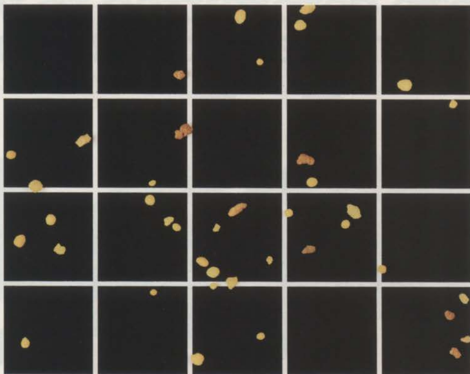
Particle distribution pattern for typical blended product.
