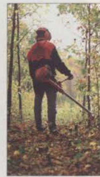
You don't have to stoop with a chain saw to thin a stand; you can simply walk along, felling trees with trunks up to 8 inches in diameter with a Husqvarna clearing saw.
