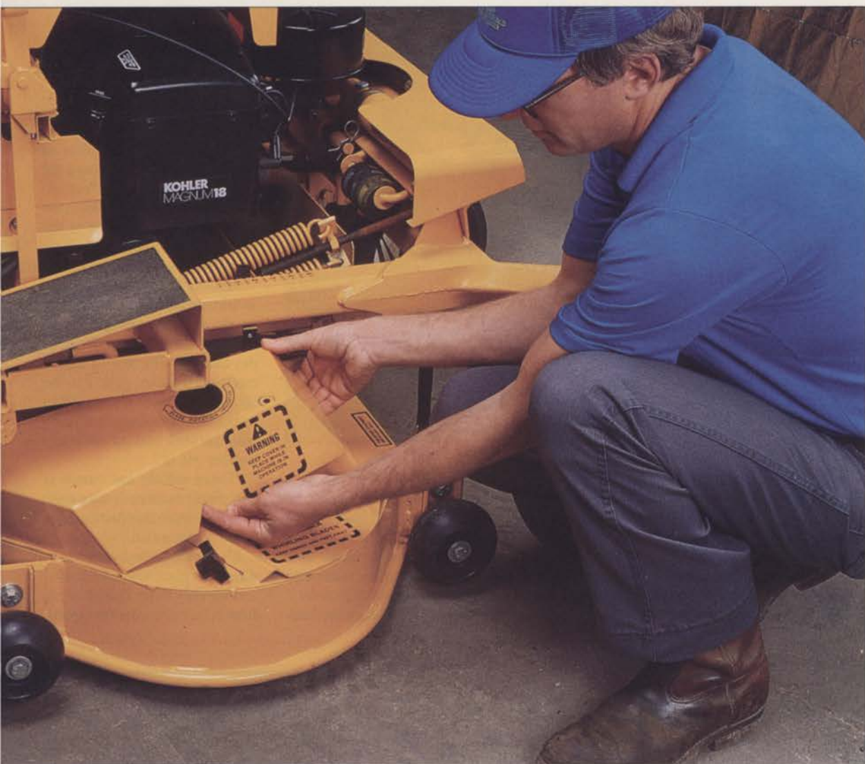
By paying attention to details, professional mowing contractors should be able to minimize the effects of equipment breakdowns. For example, keeping deck covers in place should be encouraged among your crews. Photo: Excel.
