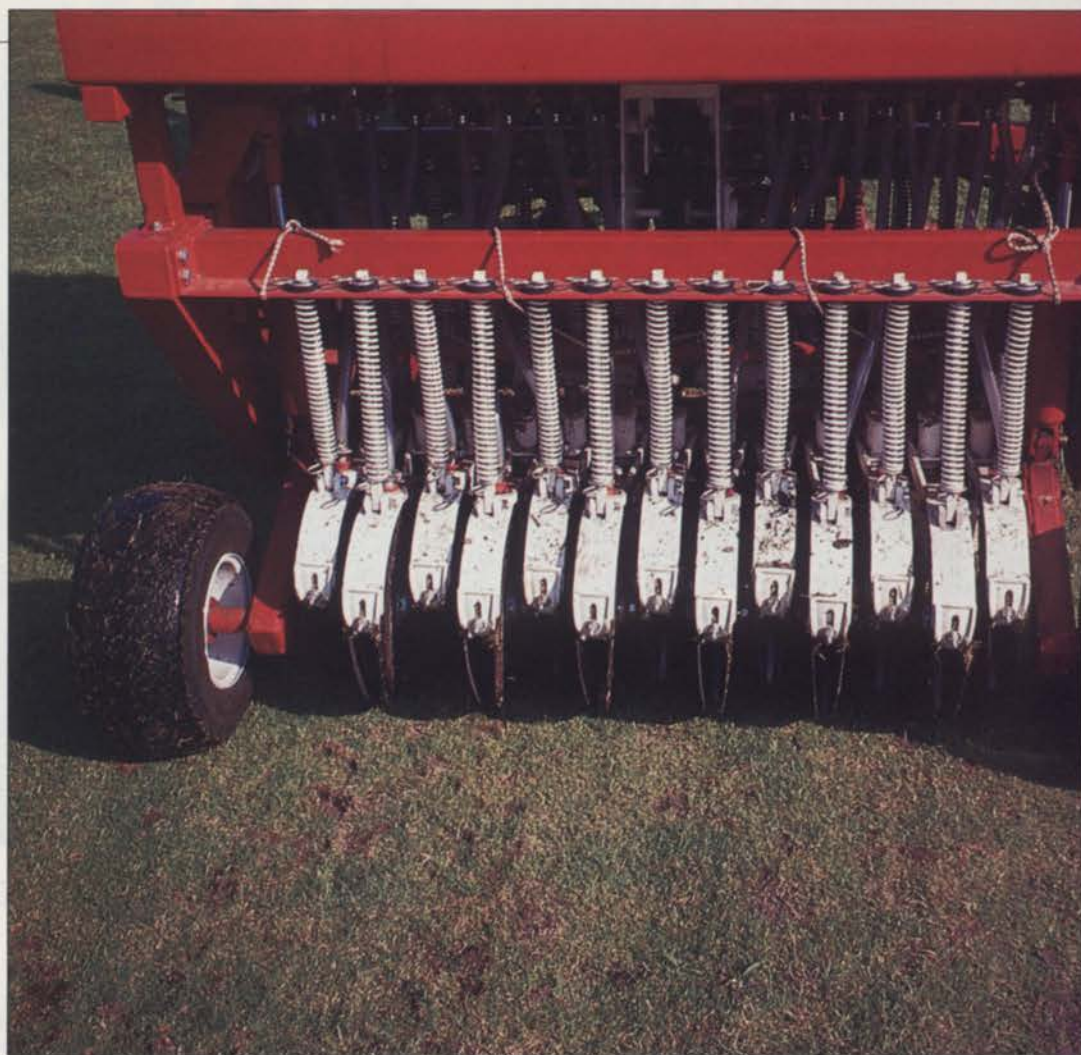
A typical design for a slit-seeder modified to inject granular formulations of insecticide. Photo: R.L. Brandenburg
