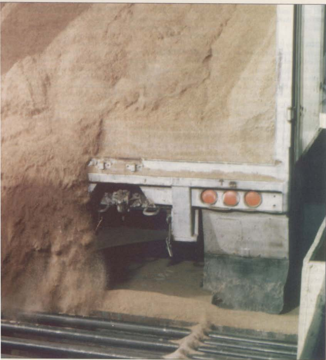
Billions of Kentucky bluegrass seeds drop into an underground receiving area to be quickly moved to cleaning machinery. Photo: Jacklin Seed.
