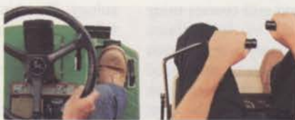
Unlike dual-lever machines, John Deere's patented hydrostatic drive gives you simple 2-pedal control of speed and direction...one forward, one reverse.
