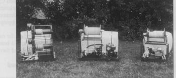
TT1050E2\* Twin Tank 2 12v Motors 2 Piston Pumps 50 & 100 Gal. PCO Tanks **TS200\* Tree Sprayer** 8 H.P. Gas Engine 14GPM Diaphragm Pump 6:1 Gear Reduction
