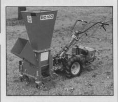
The tractor is powered by an 8-h.p. Kohler engine. A low center of gravity design provides stability on uneven terrain. All controls are handle-bar mounted for convenient operation.
