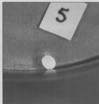
Once in liquid form, O.M. Scott's fertilizer diffuses outward through the coating.
