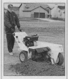
Infinitely variable hydraulic ground drive allows travel speed to be matched to digging conditions.
