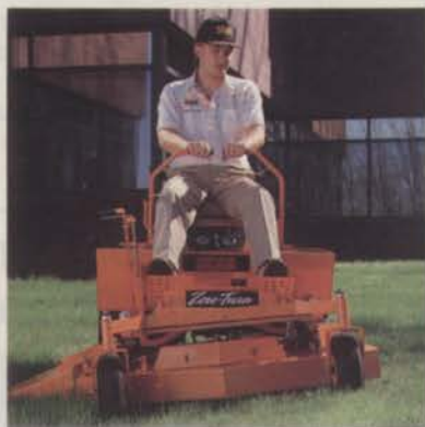
Floating articulating cutter deck provides a smooth cut on uneven turf.
