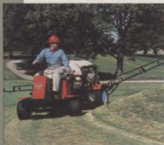
Go Boom! Independent electric controls raise and lower boom extensions
