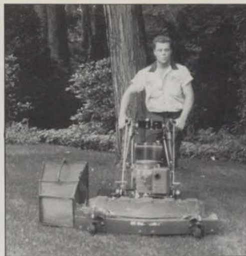
Walk-behinds offer needed versatility for mowing around landscaped areas and in other tight spots, while riders lessen operator fatigue and can make slopes easier to cut.
