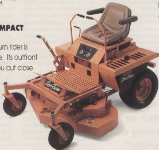
Floating articulating cutter deck provides a smooth cut on uneven turf.
