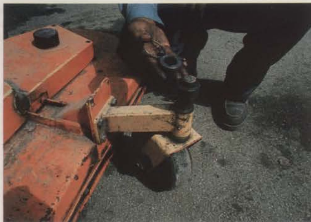
Because gasoline breaks down with time, drain the engine of old fuel before and after winter storage. Change the engine oil and filter. Clean or replace the air cleaner element and wipe out the inside cover and base. Install new spark plugs. Finally, some basic cleaning and touching up is needed. Dirt, grass and grease that is allowed to sit on surfaces during storage will lead to rust and corrosion. Photos: Clarence Davids & Sons.
