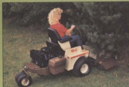
Outfront deck design lets you reach hard-to-mow areas that belly-mount mowers can't get to.
