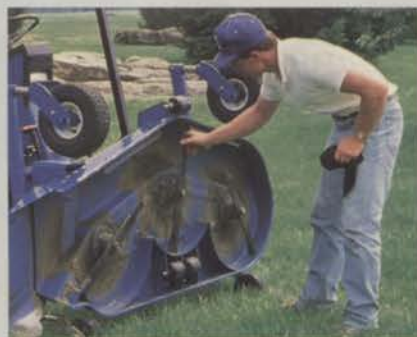
Mower deck flips up vertically for easy access. (Do not attempt maintenance while mower is engaged.)
