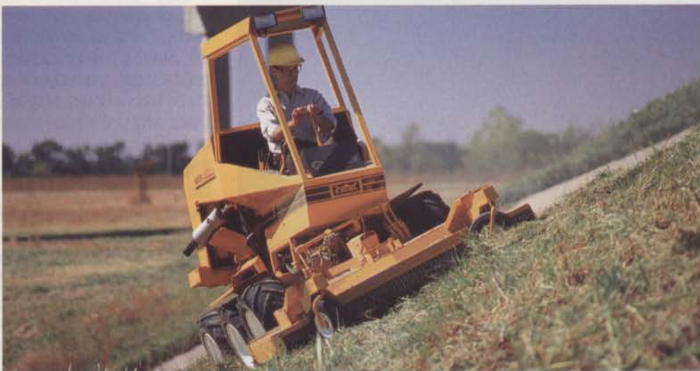
The Hustler 640 Hillsider self-levels automatically to keep driver upright when mowing on inclines.
