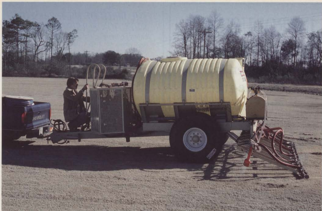
A prototype high pressure injection unit designed by Jimmy Lewis, president of Cross Equipment Co., Albany, Ga. Photo: Cross Equipment.
