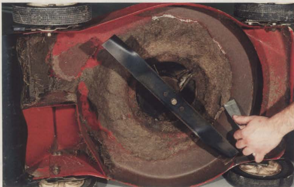
Keeping the bottom of your mower clear of dirt and corrosion, its filters clean and spark plugs free of combustion buildup adds years to mower life.
