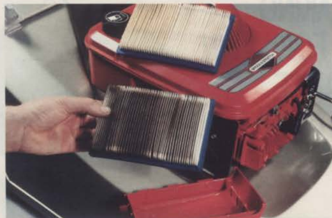
Keeping the bottom of your mower clear of dirt and corrosion, its filters clean and spark plugs free of combustion buildup adds years to mower life.
