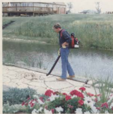
Backpack blowers are convenient for removing clippings from residential sidewalks. Photo: RedMax.
