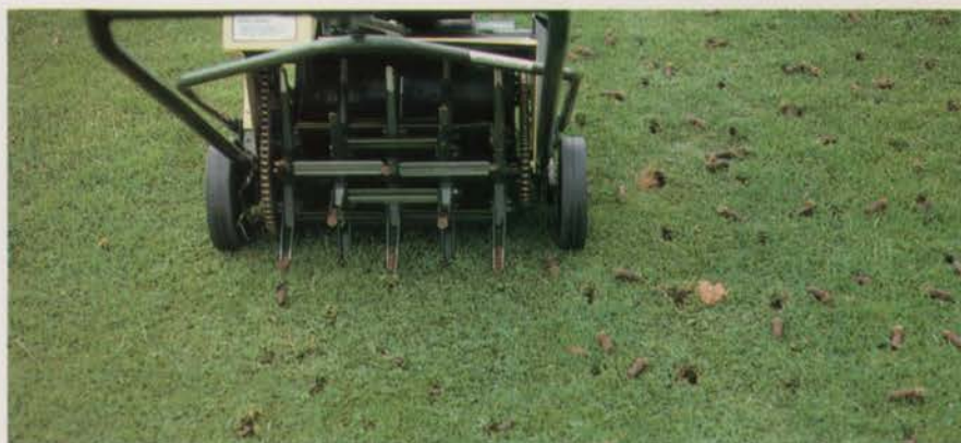
The LA 28 performs well on a variety of turf areas (top left). A visible hole pattern (below) and cores from the Lawnaire IV (top right) show the customer that a quality aeration job has been performed.
