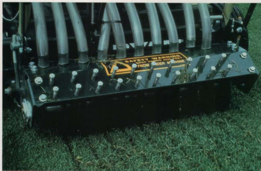
Uniform distribution and a higher seed germination can be achieved with the overseeder.
