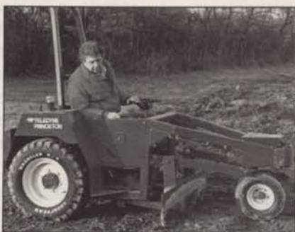
Able to turn on its own length, the Groundhog grades as close as 1/2-inch from any foundation, pipe, tree or other site obstacle. Its powerful speed and performance eliminates the need for hand raking, thereby providing substantial savings in time and labor. In addition, the product is versatile and easily converts to plow snow.
