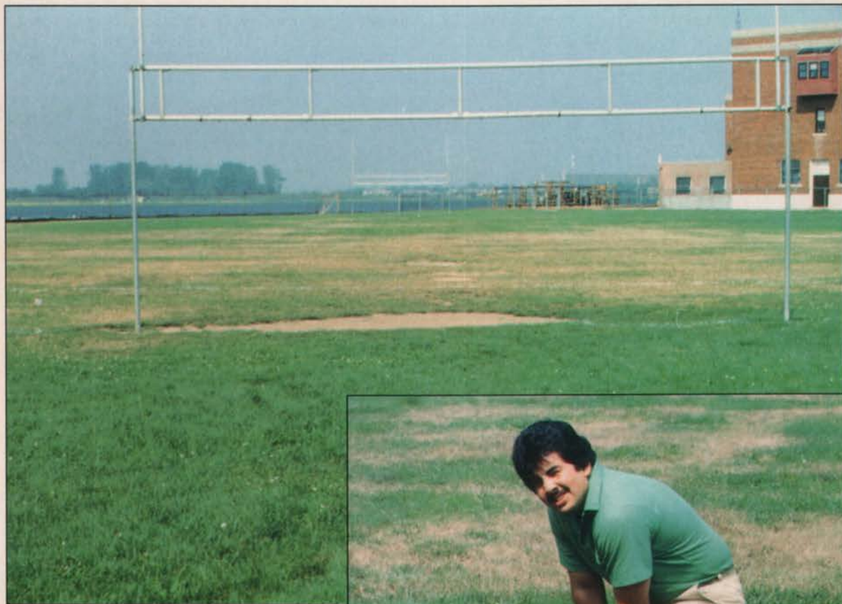
(Above) The effect of soil compaction is often evident in the poor turf appearance on the field in comparison with the area behind the goal posts. This field, supposedly ready for fall play, is hard and unfit. (Inset) When in doubt about the hardness of a sports field, insert a soil sampling tube. This soil is so dry and compact that the tube fails to penetrate more than an inch.
