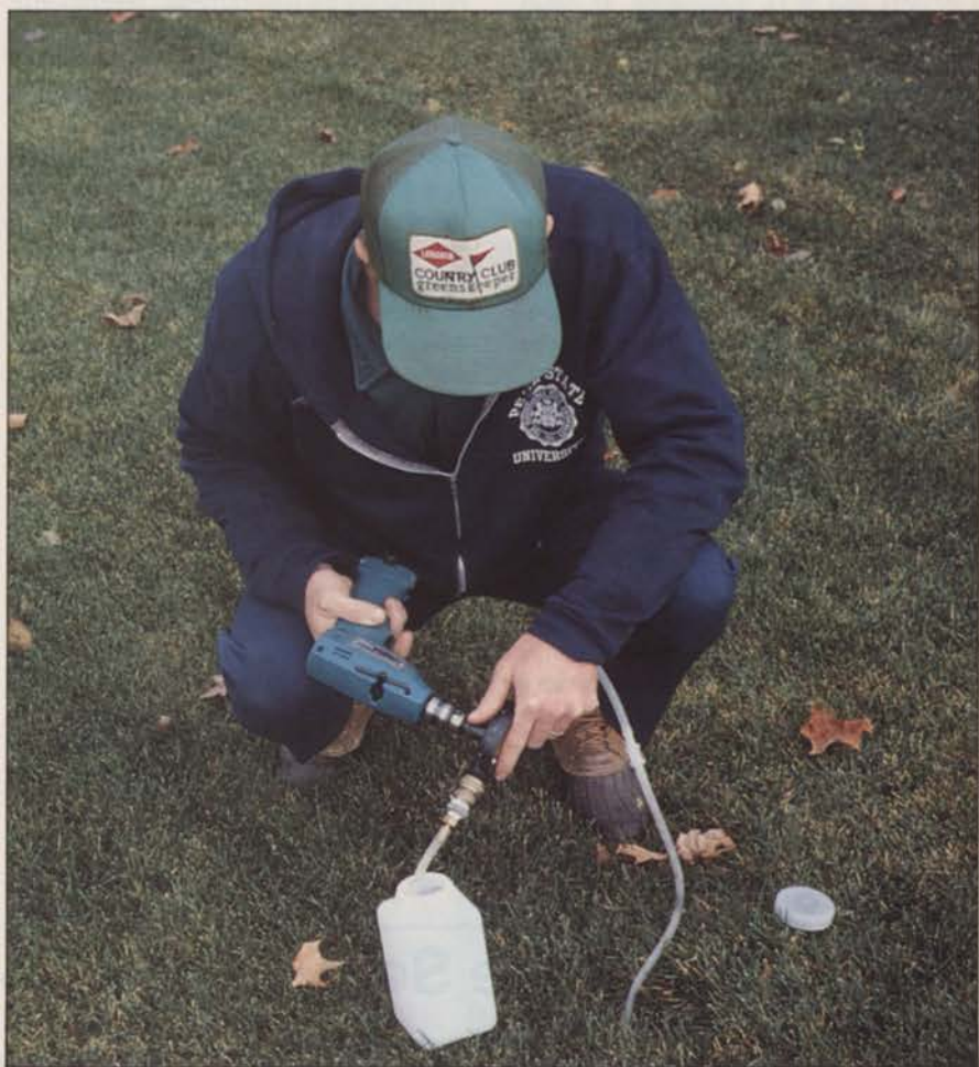
A researcher pumps out water from the underground lysimeter so he can analyze the liquid.
