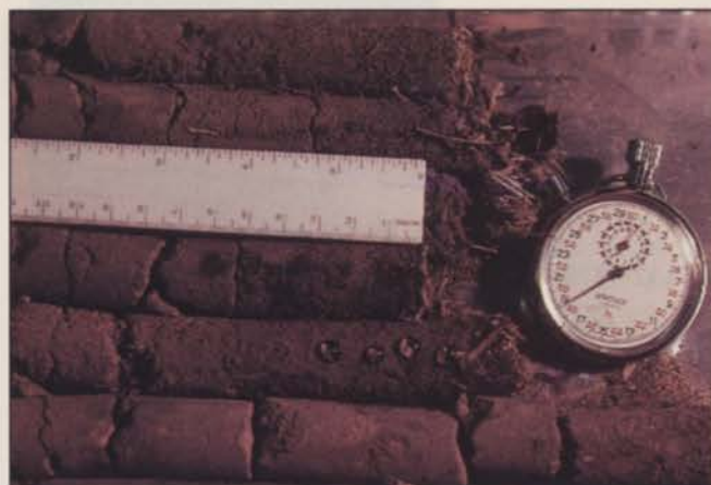
(left) The dried soil cores, treated (third from bottom) and untreated (second from bottom), were measured for hydrophobicity, based on the time required for a drop of distilled water to penetrate at various depths. (right) Soil profile showing deep silt-loam typical of alluvial deposits on the East Coast. (below) Treatments were applied using a CO 2 charged, back-pack sprayer equipped with a four nozzle boom.
