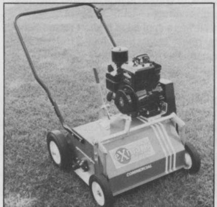
**Lawn Masters, Inc.** has added a closed spoon core aerifier to its 1987 Westmac line. With this addition, owners can convert their current Westmac from plug aerators to core aerifiers. The change is possible by either purchasing the new core aerifier assembly with closed spoons or the kit for converting an open-spooned plug aerator to that with a different weight arrangement with closed spoons.
