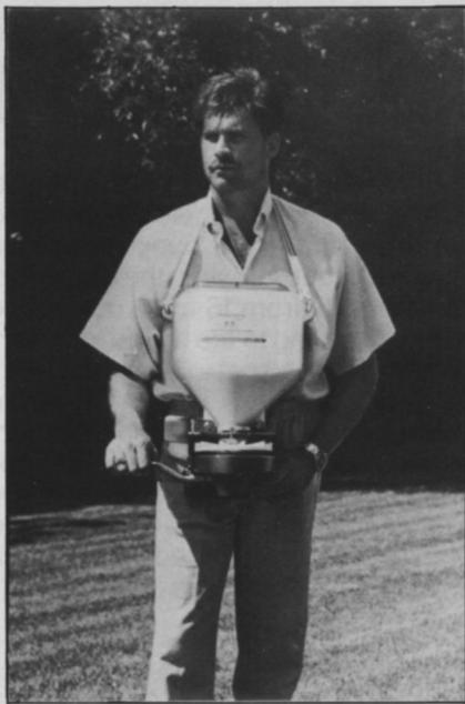
per capacity of up to 20 pounds is now available from **Warren's Turf Seed and Special Products Division**. The new spreader has a 33 percent larger hopper than the popular Warren's Model T-7 it is designed to replace. It spreads seed, pesticides, and fertilizer in paths up to 20 feet wide. It goes anywhere a person can walk because it weighs less than 6 pounds (empty) and is carefully balanced so that even when fully loaded it hangs comfor-
