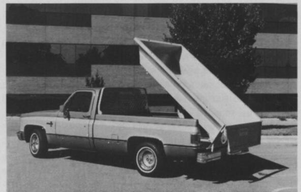
Turn your pickup truck into a multi-purpose dump truck. The Mini Dump fits most standard American pickup trucks with no modifications. The Mini Dump lifts and dumps up to 4,000 pounds and can be installed in one hour. The 600-pound carbon steel dump body insert features a high-incline dumping action, electric-hydraulic hoist and controls, all-welded construction, and a four-way tailgate. Each unit comes with a one-year limited warranty on all components and workmanship.
