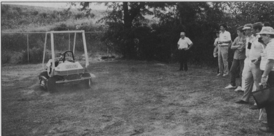
Kubota showcased its new four-wheel drive, four-wheel steering, remote-controlled mower.
