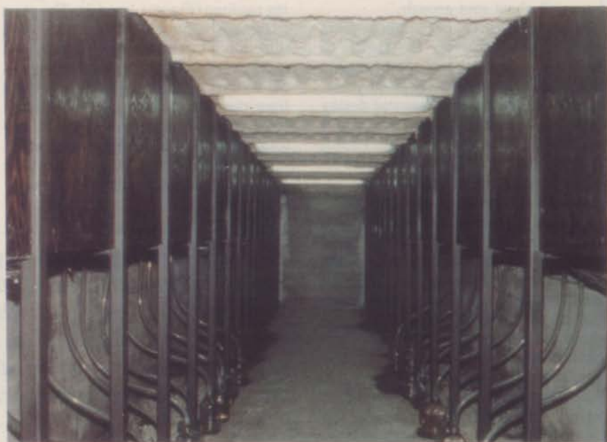
Figure 2. Below ground view of the rhizotron showing rows of rooting boxes along each side of the walkway.
