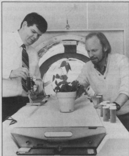
Employing a magnetic resonance scanner at GE's Research Center, Dr. Hugo Rogers (left), and Dr. Paul Bottomly are studying the structure and functioning of roots of living plants in search of ways to optimize growing conditions.
