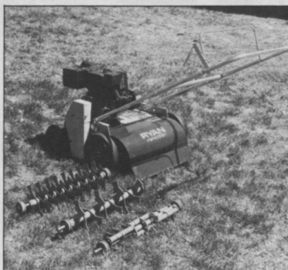
Dethatching is a step many professionals take following knock-down of the lawn with Roundup and close mowing. After the lawn is dethatched and raked off, the soil is then ready for seeding. The Ryan Ren-O-Thin is one dethatching machine on the market.
