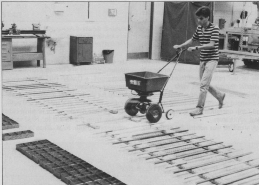
Figure 1. Laboratory test procedure showing simultaneous collection with three types of catch pans.
