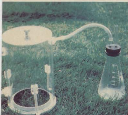
Apparatus used to trap volatile nitrogen in studies at the University of Nebraska.
