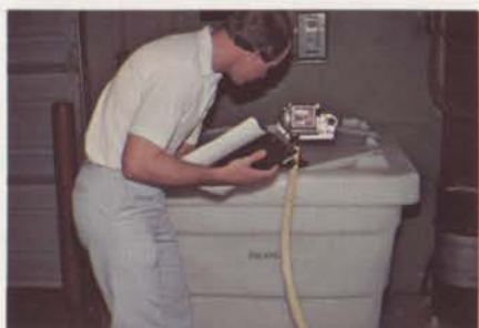
Meters with totalizers allow for accurate measurements and inventory control.
