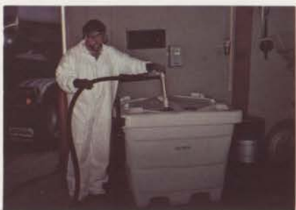
Material being dispensed at bulk tank is being metered at transporter with printed ticket for accurate measurement of delivered amount.
