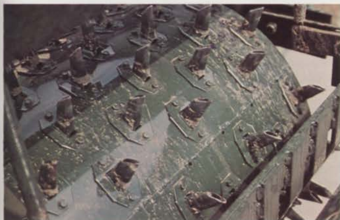
Newer type drum aerifier which provides the capability of collecting the cores. Most efficient on smaller areas.
