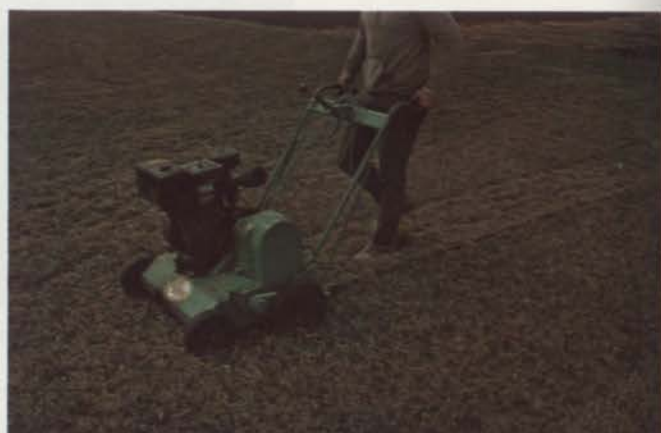
Vertical mower (Verticutter) commonly used to remove thatch from a turf.
