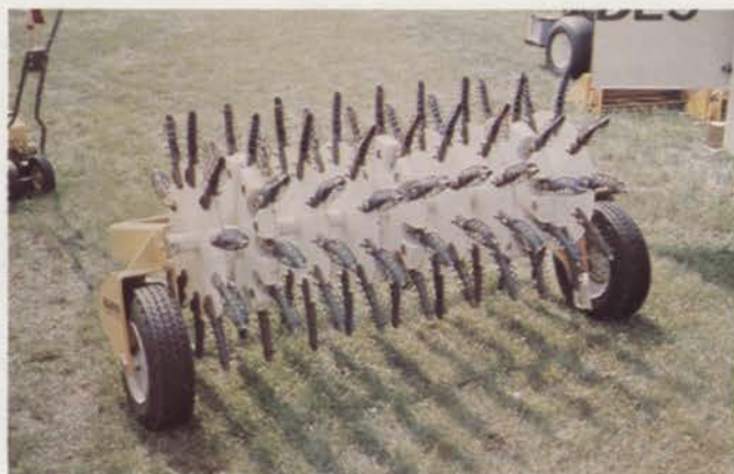
Conventional rolling tine aerifier. Type commonly used on large turf areas.
