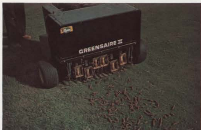
Piston type aerifier commonly used on small areas where surface disruption must be minimized.
