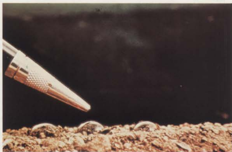
Water drops are held together by natural molecular bonds, known as surface tension. Wetting agents reduce water surface tension, encouraging more uniform water penetration and distribution.
