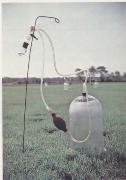
Figure 1: Apparatus used to expose field grown turf to ^{14}\text{CO}_2 . The ^{14}\text{CO}_2 is generated in the small vial glass by reacting \text{Na}_2^{14}\text{CO}_3 with lactic acid. The ^{14}\text{CO}_2 is circulated through the bell jar by means of the rubber aspirator pump.
