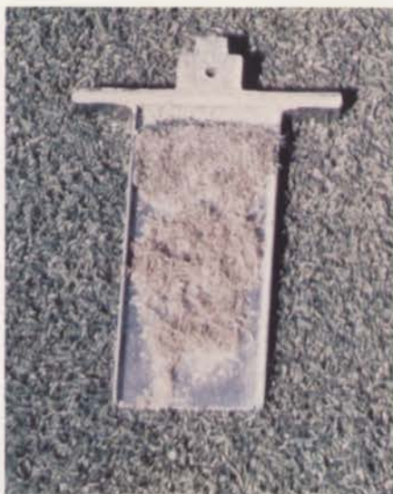
Gently wash away soil from a profile sampler to show extent of root system.
