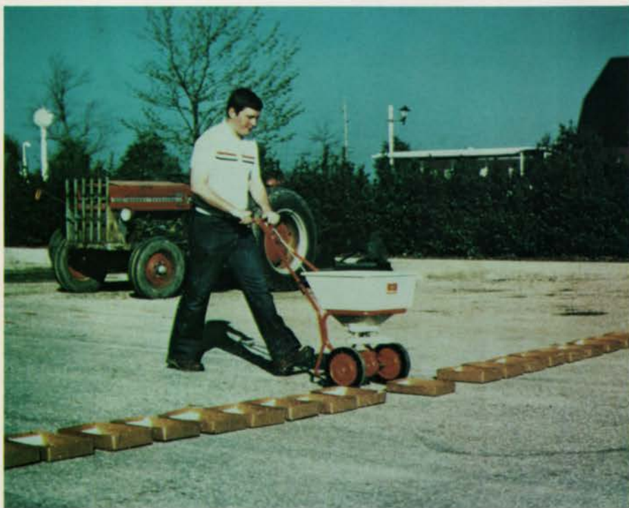
Conducting a rotary spreader pattern test.
