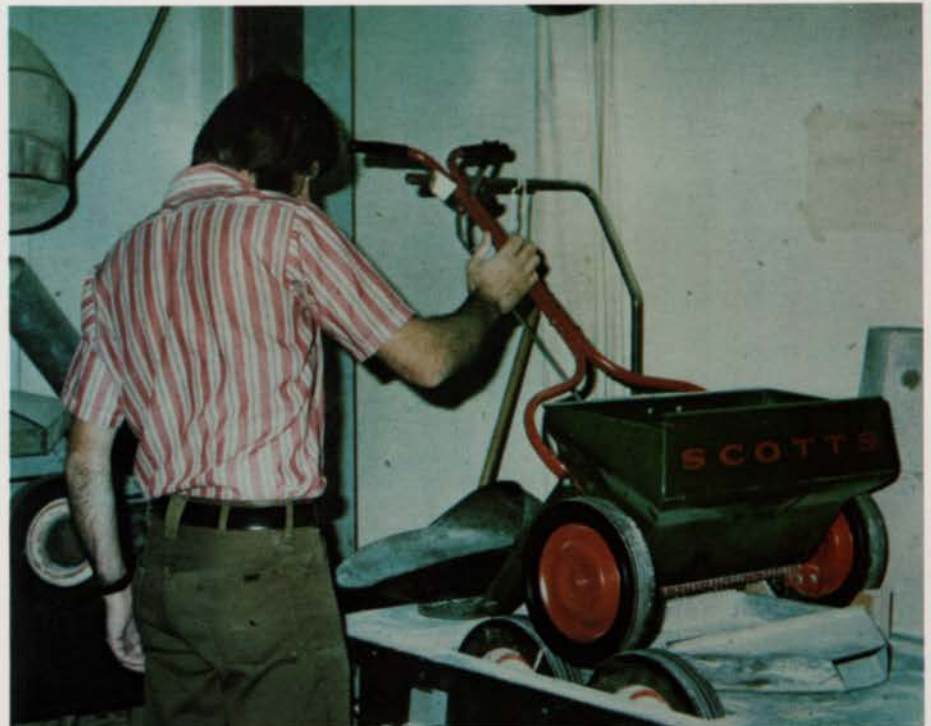
Checking spreader settings using a motorized test stand.
