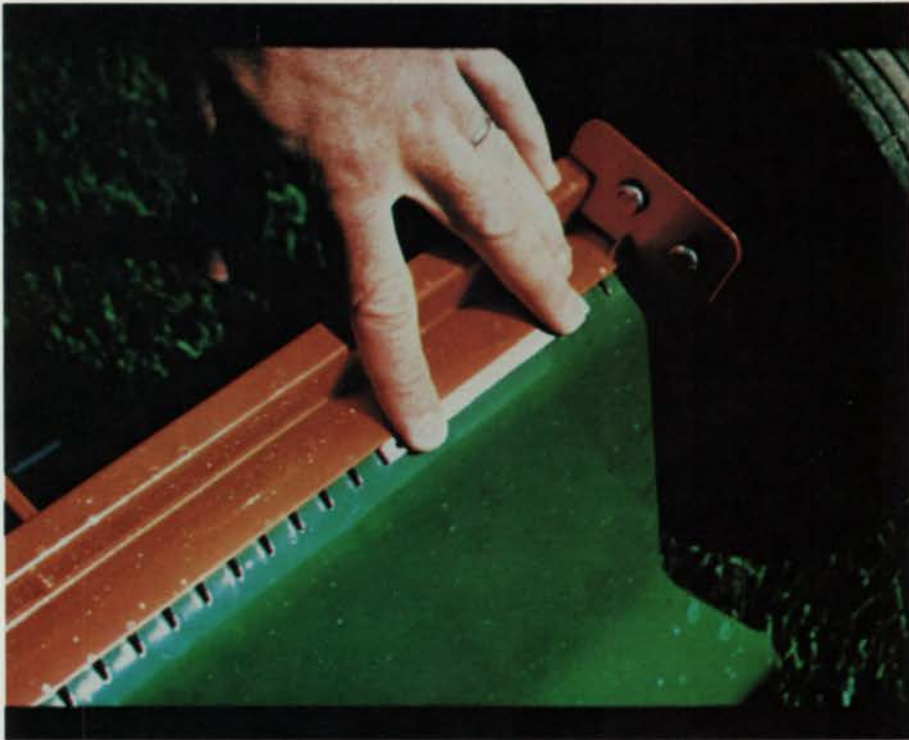
Mechanical calibration of a drop spreader using calibration gage provided by the manufacturer.
