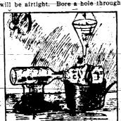
the cork. Now fill one bottle with water up to the neck (See Fig. E), then lay it over an alcohol lamp, while the other bottle (C) rests on a kitchen vessel on an exact level with the other bottle.
