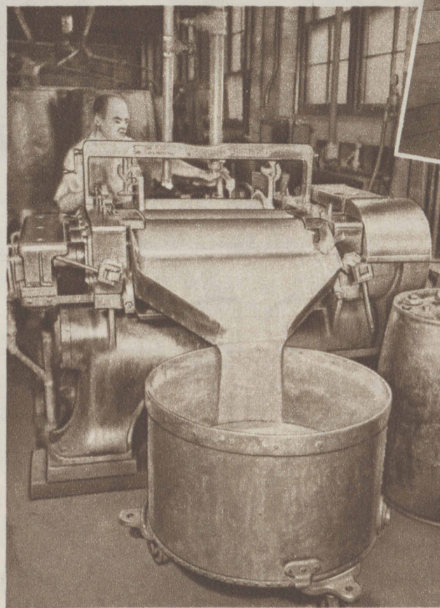
ADJACENT TO THE ROTO PLANT is the Tribune ink plant. Roto ink, unlike printers' ink, is a fluid as thin as water and contains inflammable ingredients. In this plant the Tribune now produces the best and least inflammable roto inks available and also color inks for use in Tribune newsprint color printing.
