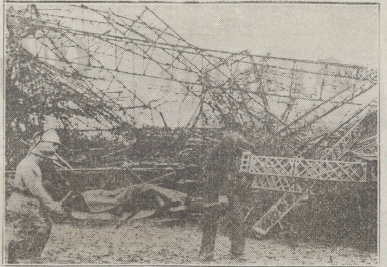
Wreckage of the giant British dirigible R-101, which crashed and exploded at Beauvais, France. It was filled with hydrogen gas.
