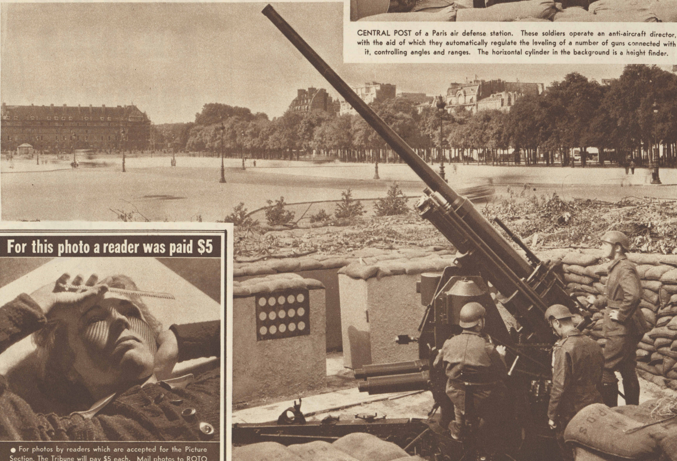
TRAINED ON THE PARISIAN SKY ABOVE THE INVALIDES—A 75 mm. anti-aircraft gun. French sources give the following data on its performance: Maximum range, approximately 14,200 yards; maximum altitude, approximately 9,800 yards. The gun is fired at the rate of twenty shots per minute.
