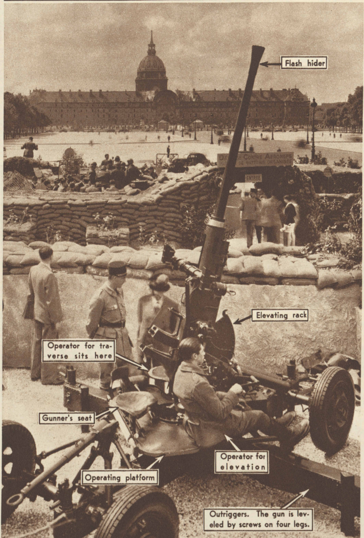
IMPORTANT IN FRENCH AIR DEFENSE, as well as English, is this 40 mm. gun made by the Bofors works of Sweden. It fires 140 shots per minute with a maximum range approaching 13,000 yards and a maximum altitude of about 5,400 yards. The 2.2 pound projectile, exploded by percussion, is said to be so sensitive that it explodes on slightest contact with a plane.
