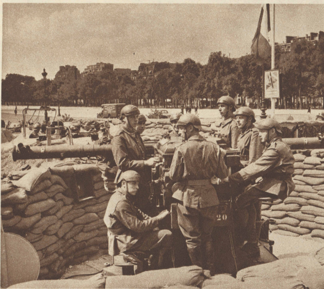
CENTRAL POST of a Paris air defense station. These soldiers operate an anti-aircraft director, with the aid of which they automatically regulate the leveling of a number of guns connected with it, controlling angles and ranges. The horizontal cylinder in the background is a height finder.
