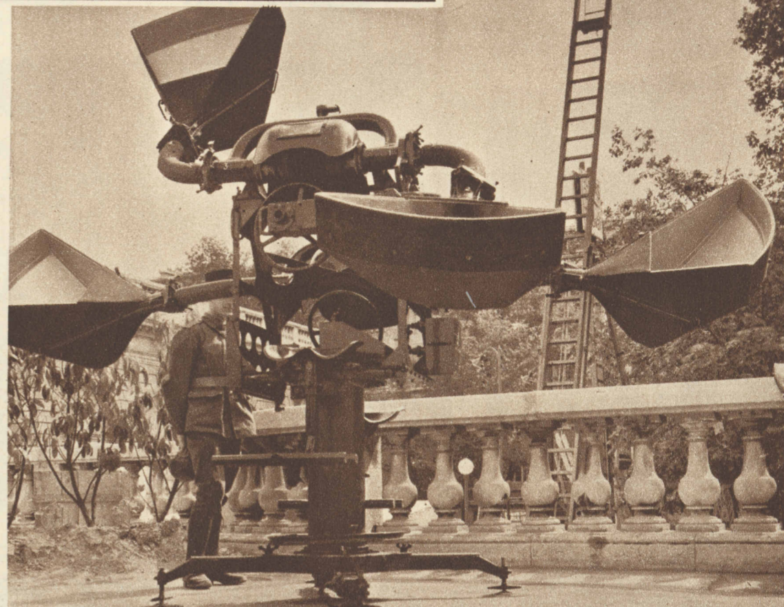
A SOUND LOCATER IN A PARIS POST—The device spot planes approaching from a distance.
