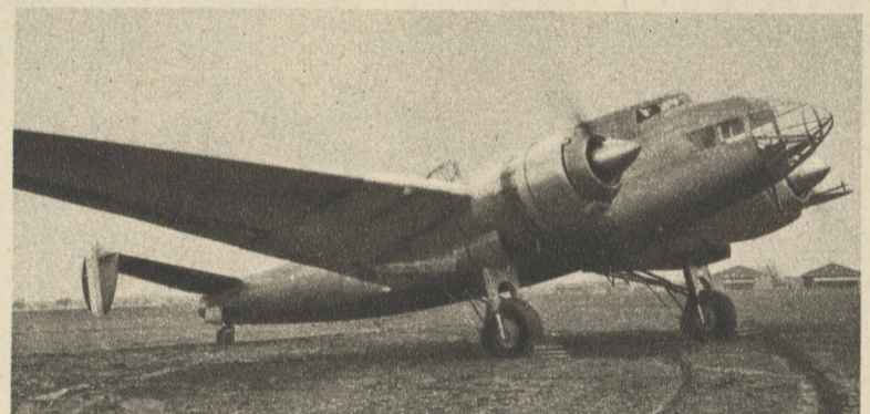
A heavy bomber capable of 311 miles an hour at 25,000 feet. It is a Leo 45.
