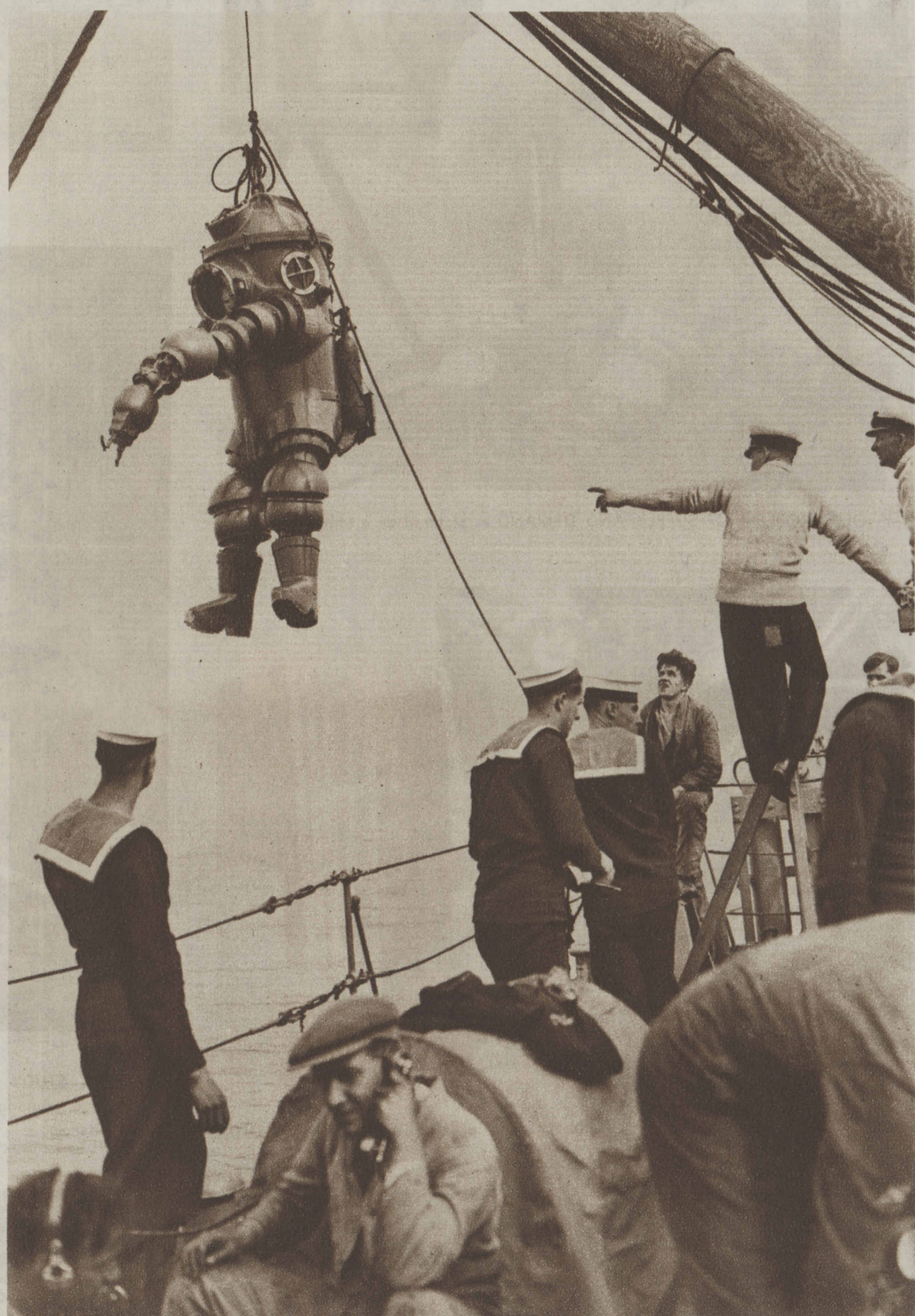
A NEW DEEP-SEA DIVING OUTFIT tested by the British admiralty. The steel diving apparatus carries its own air supply. (Acme photo.)
