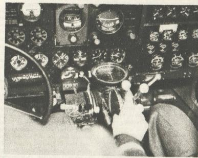
This is the apparatus through which airmen obtain bearings on radio stations from the cockpits of airliners. This particular unit is on a Transcontinental and Western Air plane. There are other types which differ only in details.
