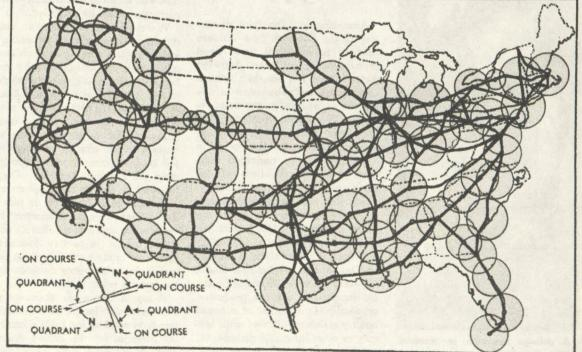
This map shows the number and location of radio beam stations in the United States. Note that most of the station zones overlap. These form the invisible roads of the gir.
